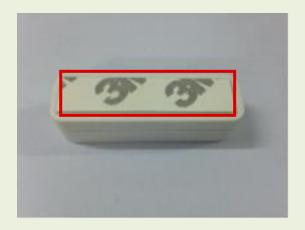
2. Tear off the 3M glue at the bottom of the reed switch probe and the magnet (as the red frame in the figure above). Then, stick the reed switch probe to the door and is parallel to the magnet (as the figure on the right).
